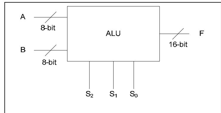
Sketch a logic circuit / block diagram to represent the ALU function above!. Assume that the C<sub>out</sub>/B<sub>out</sub> of the sum function is considered as an overflow bit
