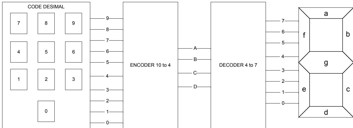
Design a circuit that can display the number on the keyboard into the 7-segment display. For example, when the number 0 on the keyboard is pressed, the display 7-segment displays the number 0. When number 1 on the keyboard is pressed, the display 7-segment will show the number 1 and so on.
