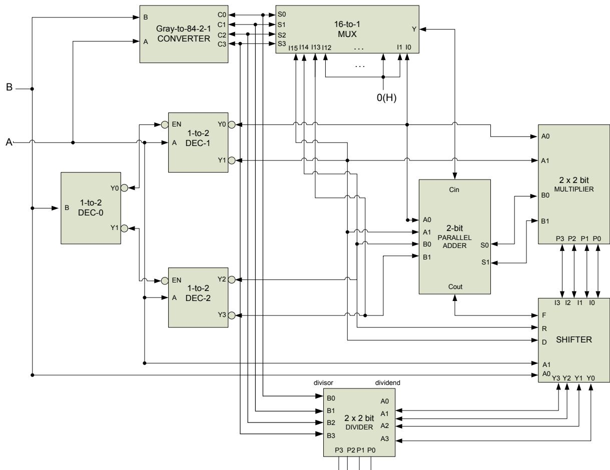
12. To make part of the ALU of a processor that can implement the required circuit Arithmetic and Logic functions in accordance with the choice of the functions assigned to the circuit as shown in the table below
