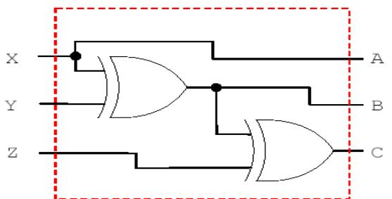
Make a truth table for logic circuit above, then give a simplified Boolean equation for each output and analysis of logic circuits what it is!
