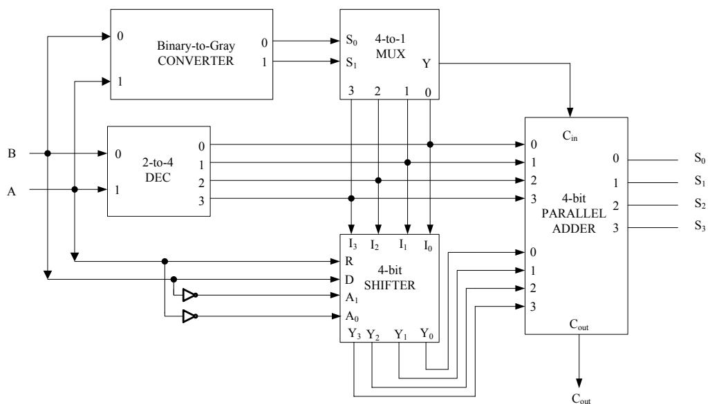
11. In the block diagram below is shown a network containing several combinational logic devices. Complete the following truth tables.
