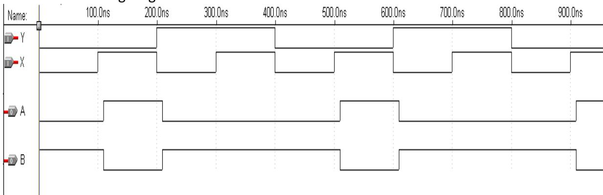
In the picture above, X and Y are the input variables while A and B is the output variable. Make a truth table of the timing diagram above then write the Boolean function of its
